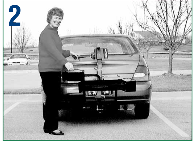
2 Lift lever and fold down platform.
