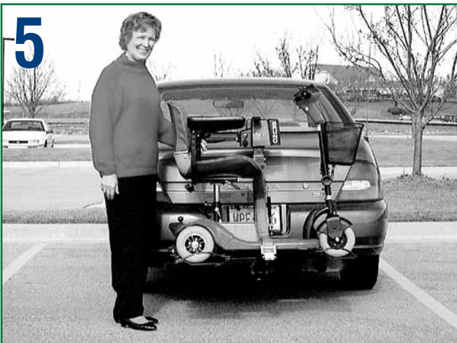
5 Roll scooter on platform, press switch to raise and secure with belt.
