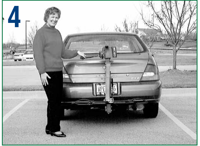
4 Press switch to lower platform.
